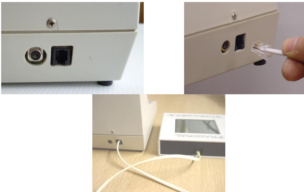
Figure 3 - Branchement du câble RJ11
