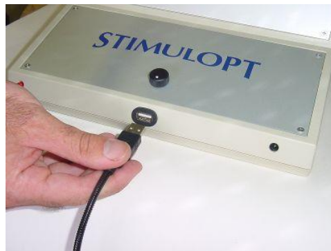
Figure 2 - Branchement du flexible USB
