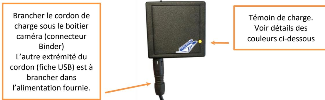
**Figure 12 - La charge du Framiscope**
