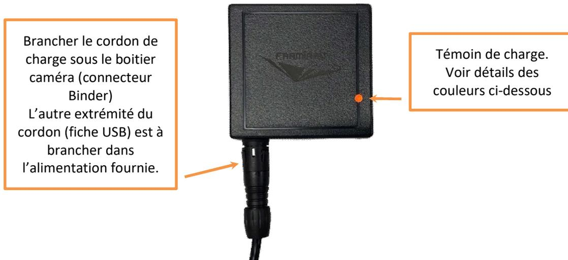
**Figure 12 - La charge du Framiscope**
